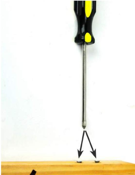
**Step 4:** Securely hold the Wooden Rack Foot (B) to the Wooden Rack (A) and using Small Philips Screw Driver, screw the Screws (C) until the screws pierce into the bottom of the Wooden Rack (A) and securely hold in place. Repeat this step for the other Wooden Rack Foot (B).
