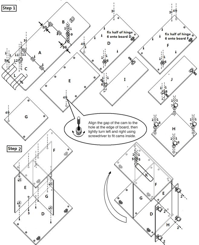
2. Insert Cam bolt (3) on board D into the Cams (4) on board E and G as shown above, turn the cams clockwise. Insert Cam bolt (3) on board F into the Cams (4) on board E and G, turn the cams clockwise. Use screw (1) to connect Caster (7) and Locking Caster (8) onto board H.
