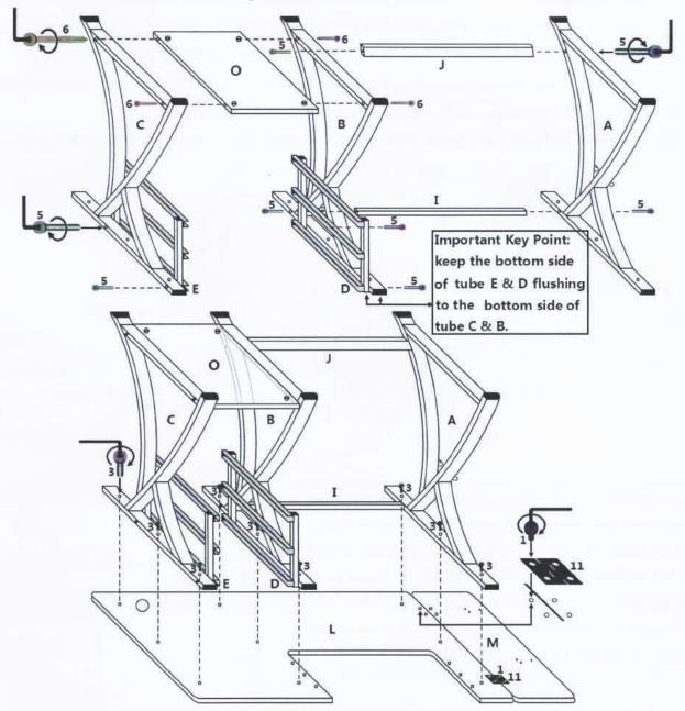
Step 2A, Use part #1 Screw to screw the part #11 Hinges onto Table Top L & M, use part #3 Screws to screw
