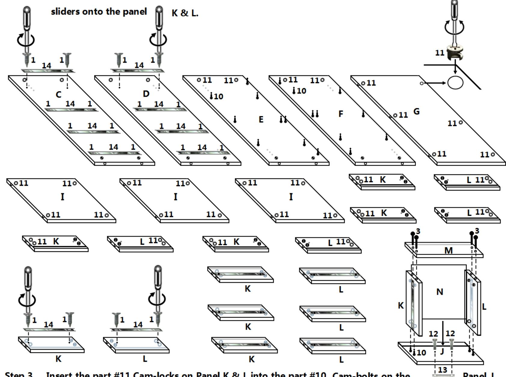
Step 3, Insert the part #11 Cam-locks on Panel K & L into the part #10 Cam-bolts on the insert panel N into the slots of panel K, L and J, and tighten these Cam-locks clockwise. Use part #3 Screws to screw the panel M with panel K & L, use part #12 Screw to screw the part #13 onto panel J.
